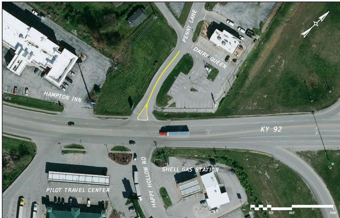
Figure 7: Right In / Right Out Penny Lane Configuration (Option B)
