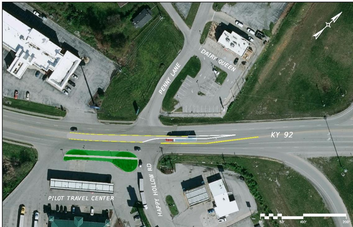
Figure 8: Proposed KY 92 & Penny Lane Intersection Configuration (Option C)
